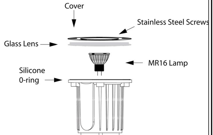
**Important:** Do not attach the cover screws too tightly into the cover. Allow a very small space between the cover and the housing. Attaching the cover too tightly to the housing may damage the glass lens.
